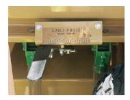
The easy one-lever calibration sets all of the seed cups to the desired seeding rate. Seed calibration rates can be further expanded with easy drive chain configuration.
